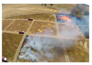
Figure 1. Aerial view of simultaneous paired experiments to examine the effect of different curing states on fire behaviour. The fire at top right is in fully cured grass whereas the fire in the foreground is in 60% cured grass.
